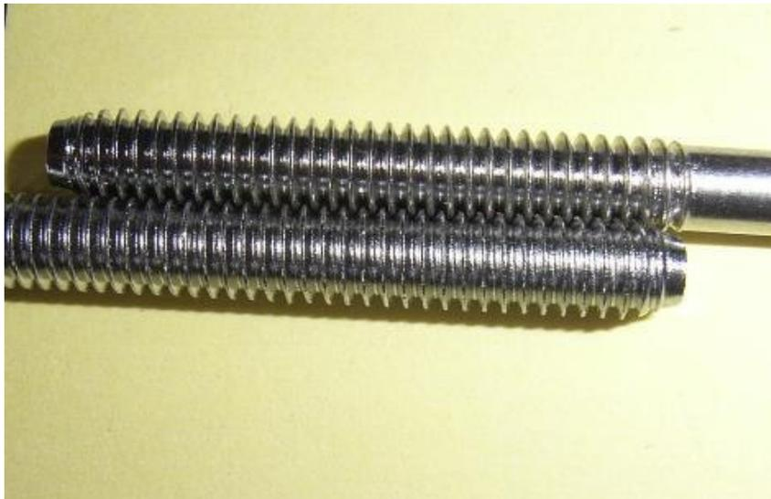
Or use a screw you be sure about the thread and hold it on the unknown screw like the picture shows. If its threads fit in like in the picture and the diameter is the same you are sure to have the same thread
